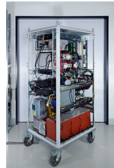
Flexible Power System Simulator (FlePS) for PHIL experiments at RWTH ACS Lab.
