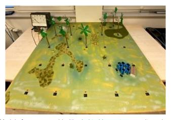
Figure 2-44 – Model of an energy grid with wind turbines, storage units and consumer LED's
